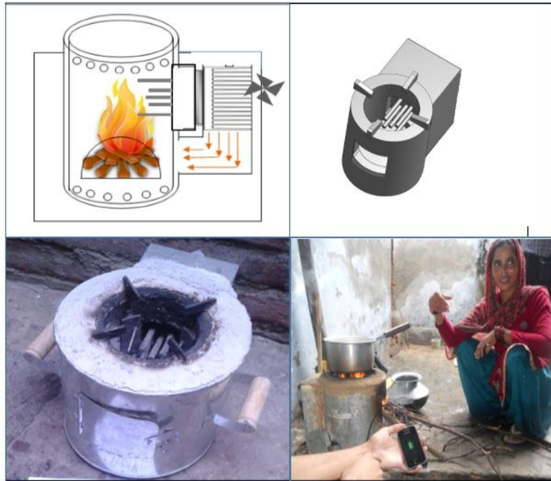
A. Conceptual Design of TEG Biomass Cook stove; B. CAD Design of TEG Biomass Cook stove; C. Actual Design of TEG Biomass Cook stove; D. Field testing of TEG stove
